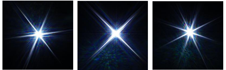
Fig. 2: Diffraction patterns of triangular, rectangular and octagonal aperture
